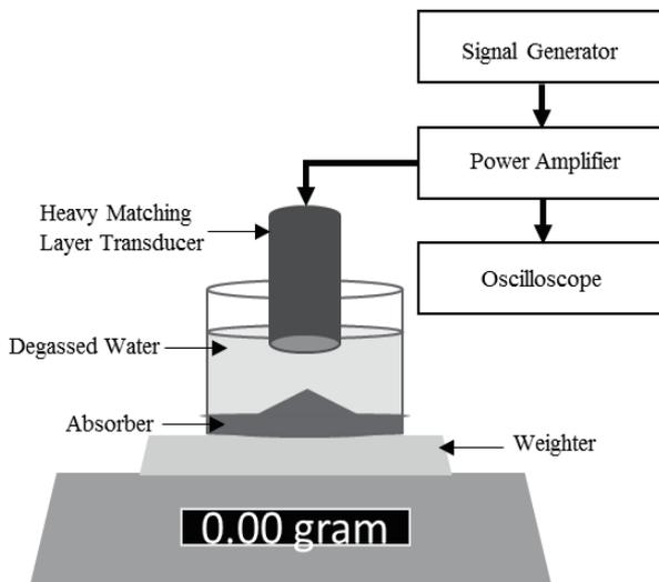
Fig. 4. Schematic of experiment setup.
