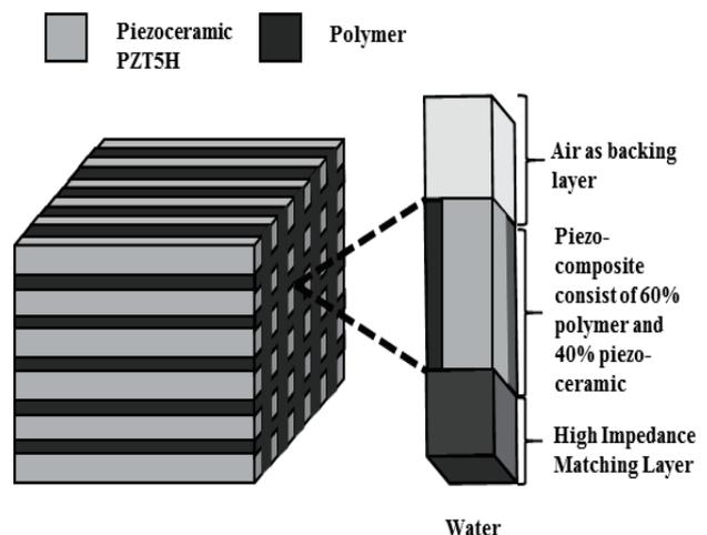
Fig. 2. Numerical model design.
