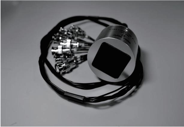
Fig. 3. Heavy matching layer prototype transducer.
