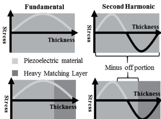
Fig. 1. Effect of heavy matching layer on fundamental and second harmonic.
