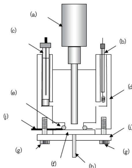
Figure 1. Schematic diagram of the ultrasonic ECL cell. (a) ultrasonic transducer, (b) Pt counter electrode, (c) Ag/AgCl reference electrode, (d) Teflon blocks, (e) o-ring, (f) ITO working electrode, (g) screws, (h) optical fiber, (i) Teflon plate and (j) copper foil.
