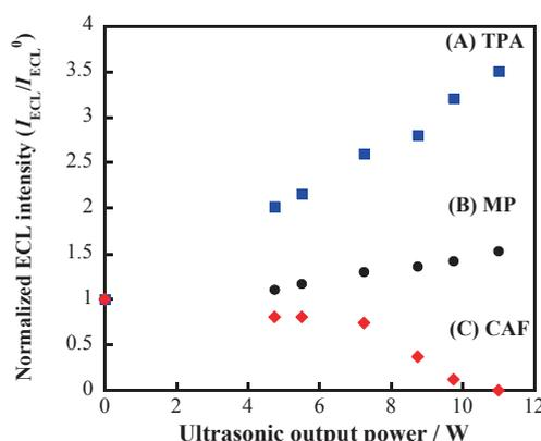
Fig. 3 Effect of the ultrasound output power on ECL enhancement factor ( $I_{ECL}/I_{ECL}^0$ ) in Ru(bpy)<sub>3</sub><sup>2+</sup> based ECL systems using (A) TPA, (B) MP and CAF as co-reactants, respectively.
