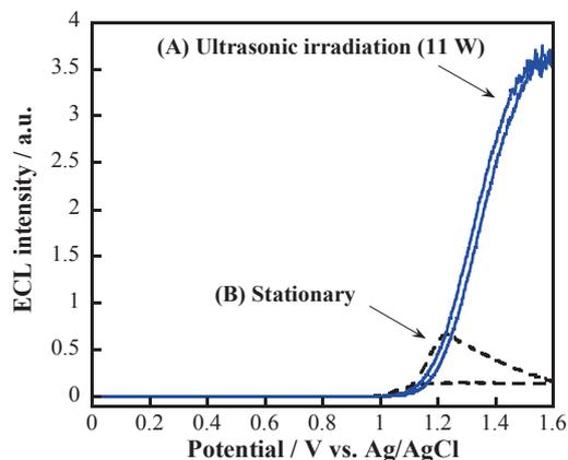
Fig. 2 ECL responses for 0.50 mM Ru(bpy)<sub>3</sub><sup>2+</sup> and 0.50 mM TPA in 0.1 M phosphate buffer solution (pH 9.0) at ITO electrode. (A) with sonication (solid line) and (B) stationary condition, respectively.
