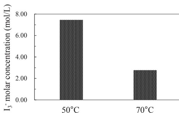
Fig. 3 I<sub>3</sub><sup>-</sup> molar concentration in the solutions irradiated at 50 or 70°C (I<sub>3</sub><sup>-</sup> generated was calculated using KI method.)
