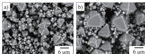
Fig. 2 SEM images of scorodite particles at 70°C using a) stirring and b) ultrasound.
