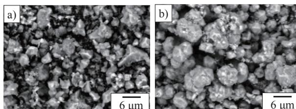
Fig. 1 SEM images of scorodite particles at 50°C using a) stirring and b) ultrasound.
