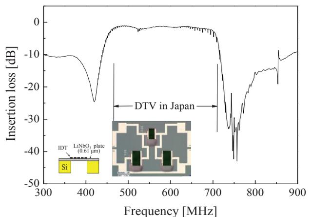
Fig. 3 T-type ladder filter device and the frequency characteristic with WR of 1.39.
