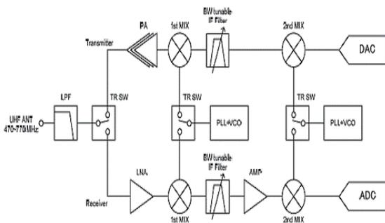
Fig. 1 Block diagram of up-conversion-type RF Front-end for IEEE802.11af using bandwidth tunable filters.
