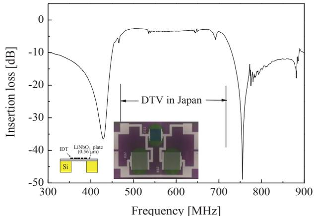
Fig. 5  $\pi$ -type ladder filter device and the frequency characteristic with WR of 1.43.
