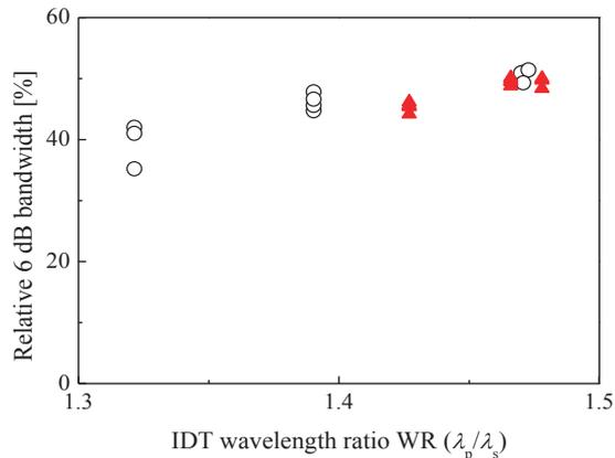
Fig. 4 6 dB BWs of ladder filters as a function of WRs. The white circles and the red triangles represent BWs of T-type (AR=0%) and  $\pi$ -type (AR=60%) ladder filters, respectively.
