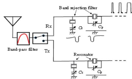
Fig. 2 Block diagram for cognitive radio system using ultra-wide band-pass filter covering fully DTV band and band rejection filters.
