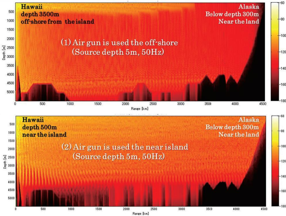
Fig3. Air gun signal propagation sound field from Hawaii to Alaska
