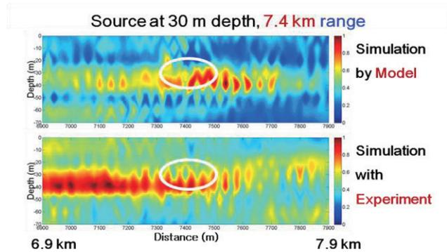
Fig. 8. Sound refocusing to source location by time reversal technique at source target depth 30 m, 7.4 km range.
