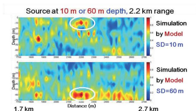
Fig. 9. Comparison for sound refocusing simulation about two source depth(10 m and 60 m) by time reversal technique at source target depth 30 m, 2.2 km range.
