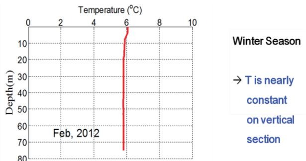
Fig. 3. Water temperature measured by CTD in shallow water.
