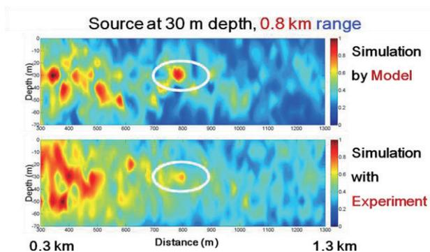
Fig. 5. Sound refocusing to source location by time reversal technique at source target depth 30 m, 0.8 km range.
