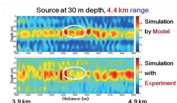
Fig. 7. Sound refocusing to source location by time reversal technique at source target depth 30 m, 4.4 km range.
