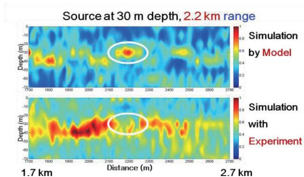
Fig. 6. Sound refocusing to source location by time reversal technique at source target depth 30 m, 2.2 km range.
