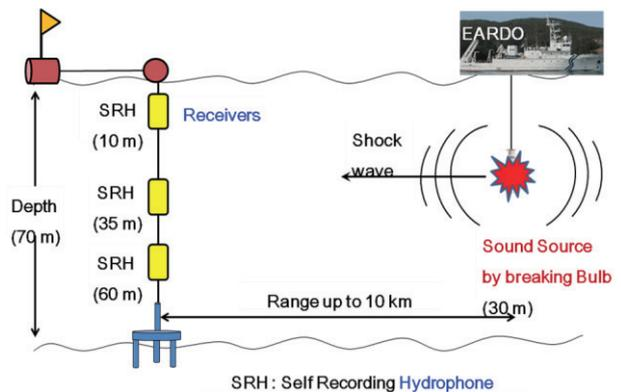
Fig. 2. Schematic diagram of time reversal acoustic experiment in shallow water.
