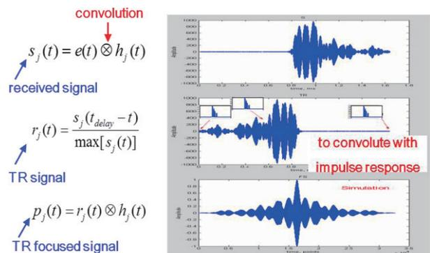
Fig.1. Principle of time reversal technique.
