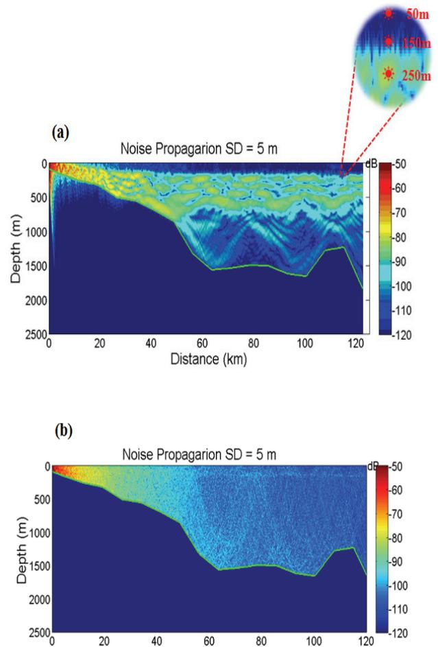
Fig. 3 Propagation losses of shipping noises at the frequencies of 100 Hz and 1 kHz in the coastal sea.
