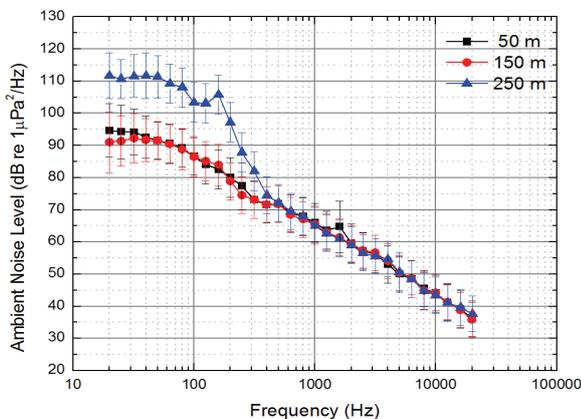
Fig. 2 Mean noise levels of ambient noises observed at the experimental site.
