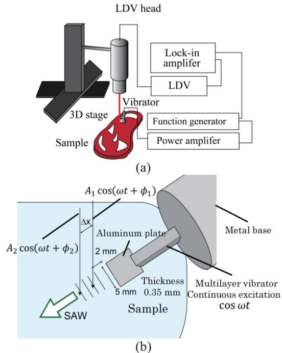
Fig. 1. Experimental setup: (a), Overview; (b), Close up of the vibration exciter.
