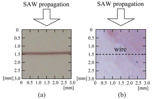
Fig. 4. Photos of the samples: (a), Agar sample with lead wire; (b), Pork sample with lead wire.
