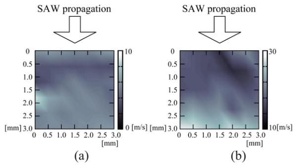
Fig. 5. 2D SAW velocity mapping: (a), Agar sample with lead wire; (b), Pork sample with lead wire.
