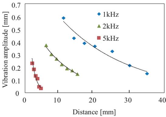
Fig. 3. SAW attenuation in the 2% agar sample.
