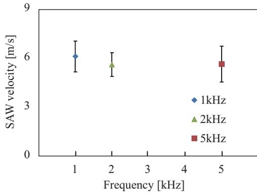
Fig. 2. SAW velocity in the 2% agar sample.
