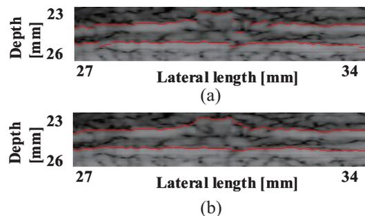
Fig. 5. Detected boundaries of arterial wall mimicking phantom by (a) the simple method and (b) the proposed method
