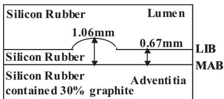
Fig. 3. Structure of the phantom mimicking the arterial wall.
