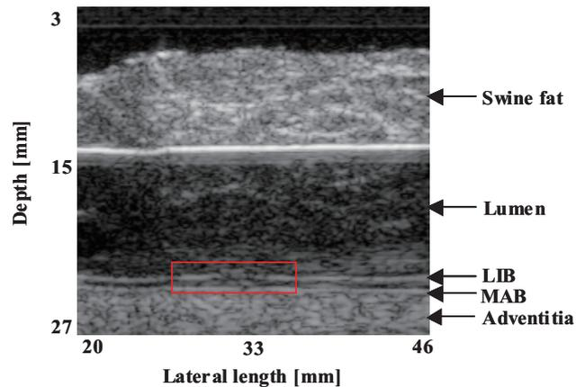
Fig. 4. B-mode image of arterial wall mimicking phantom on which swine fat layer is located
