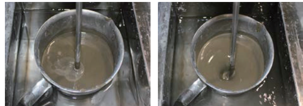
Fig.4 Flowability change due to ultrasonic energy
