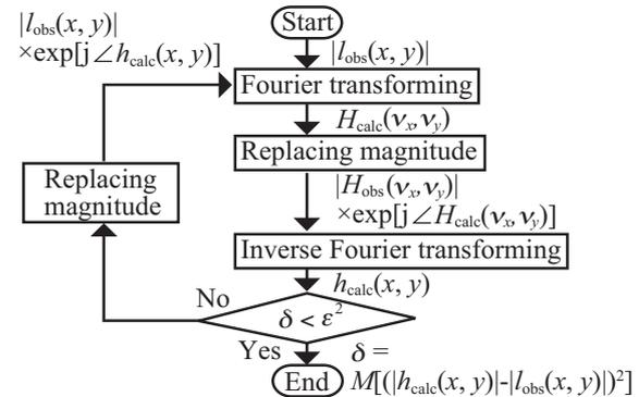
Fig. 2 Fourier iterative phase retrieval.
