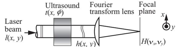
Fig. 1 Optical Fourier transform.
