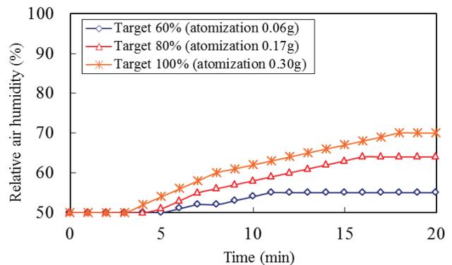
Fig.2 Change in relative air humidity by atomization at 10°C.
