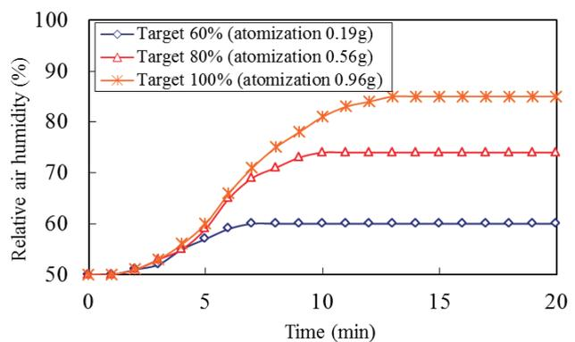
Fig.3 Change in relative air humidity by atomization at 30°C.
