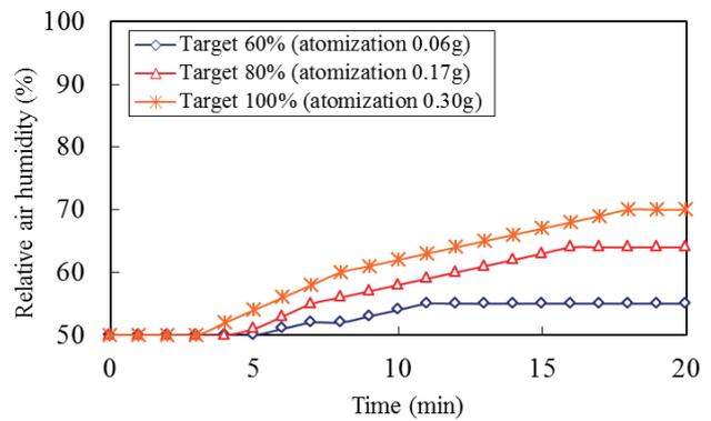
Fig.2 Change in relative air humidity by atomization at 10°C.
