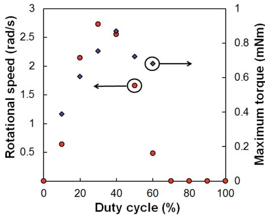
Fig. 4 Rotational speed and maximum torque as functions of duty cycle.
