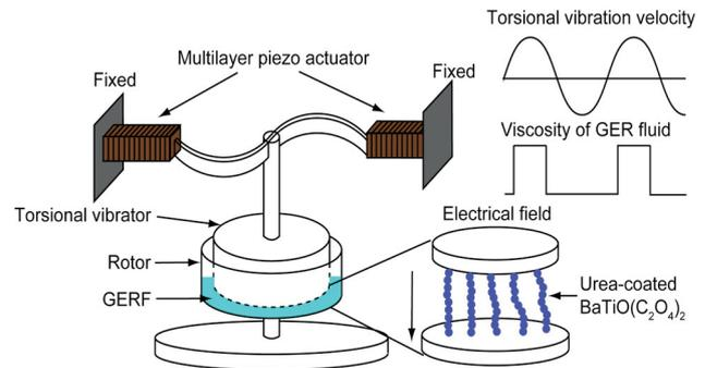
Fig. 1 Configuration of the prototype piezoelectric motor using torsional vibrator and GER fluid.
