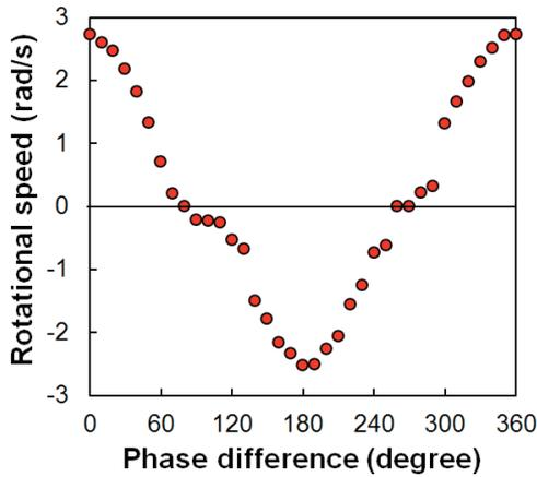
Fig. 2 Dependence of the rotational speed on the phase difference between the electric field applied to GER fluid and the torsional vibration velocity.
