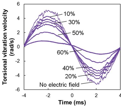
Fig. 3 Dependence of the torsional vibration velocity on duty cycle.
