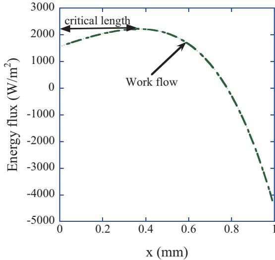
Fig. 1 The result of the numerical simulation on the work flow as a function of  $x$  in a stack.
