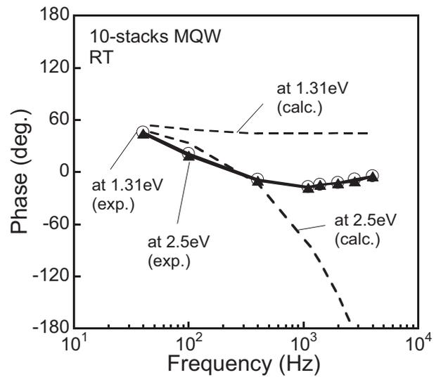
Fig. 2 The theoretical and experimental phase as a function of the chopping frequency
