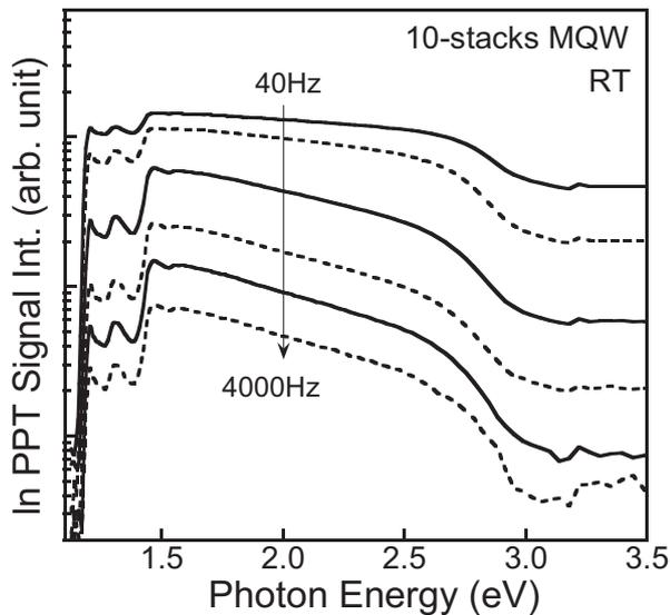
Fig. 1 The chopping frequency dependence of the PPT spectra at room temperature
