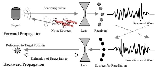
Fig. 1 Approach for target range estimation using ANI system with acoustic lens.
