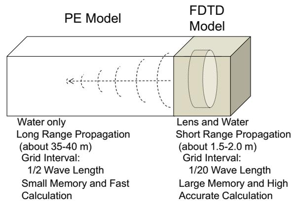
Fig. 4 3D volume of analysis domain of numerical calculation for backward propagation.
