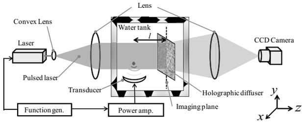
Fig. 2 Optical measurement setup.
