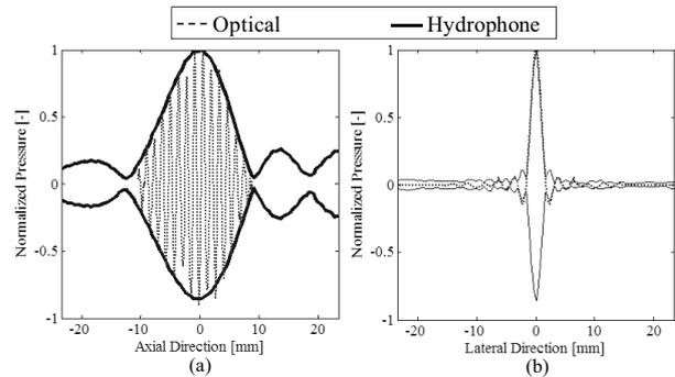
Fig. 3 Comparison between two methods for  $l=40$  mm. (a) axial direction, (b) lateral direction.
