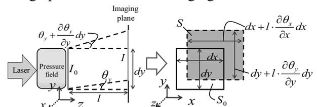
Fig. 1 Intensity modulation due to phase variation.
