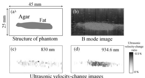
Fig.2 Phantom structure for preliminary experiment and ultrasonic images obtained by light irradiation with 0.830nm and 0.935nm.
