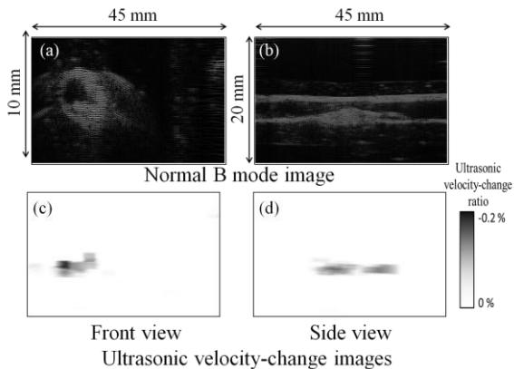
Fig.5 B mode images and ultrasonic velocity-change images obtained by ultrasonic warming
