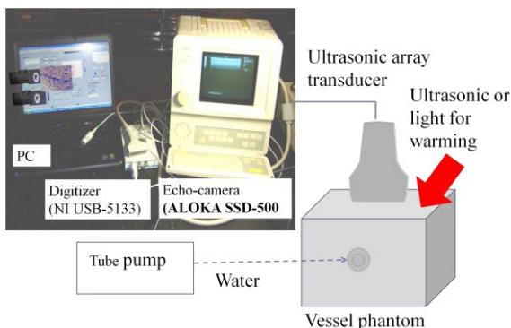
Fig.1 Experimental set-up for constructing the ultrasonic velocity-change image of vessel phantom
