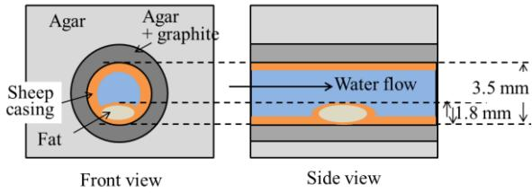
Fig.3 Structure of vessel phantom made of sheep intestines and agar
