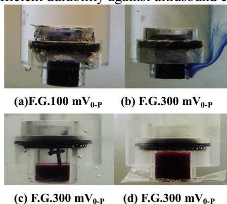
Fig. 3 Observation of damage of our fabricated cell flask by ultrasound irradiation (a)(b)fabricated by heat welding(PMMA body and OPS film), (c)fabricated by ultrasound welding(PET body and OPS film), (d) fabricated by ultrasound welding(PET body and Lumirror film)
