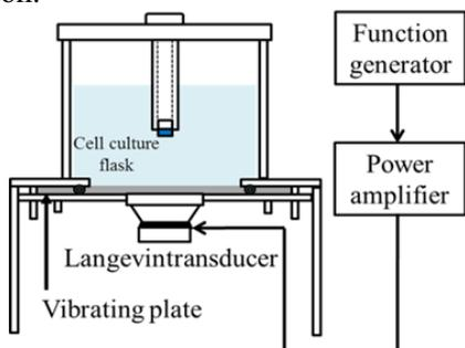
Fig. 2 Block diagram of ultrasound irradiation system for our fabricated cell flask with acoustic window film
