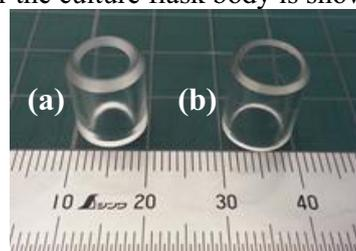
Fig. 1 Photograph of the resin pipes for the culture flask body (a) PMMA, (b) PET
