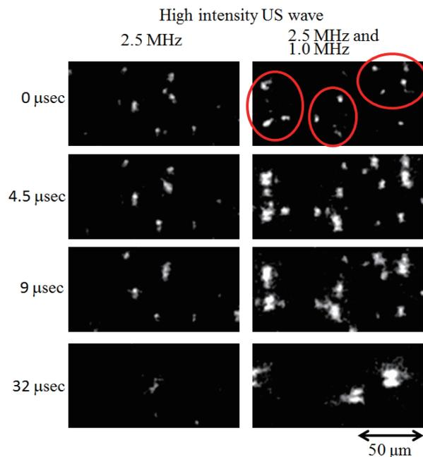
Fig. 3 Bubble clouds when high intensity US wave with two frequencies of 1.0 MHz and 2.5 MHz irradiates.
