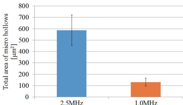
Fig. 2 Total area of micro hollows when high intensity US waves of 2.5 MHz and 1.0 MHz irradiate.
