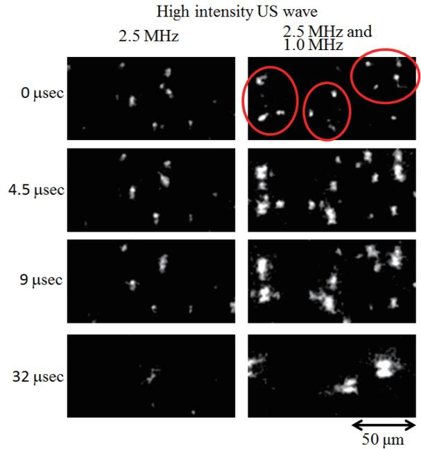
Fig. 3 Bubble clouds when high intensity US wave with two frequencies of 1.0 MHz and 2.5 MHz irradiates.
