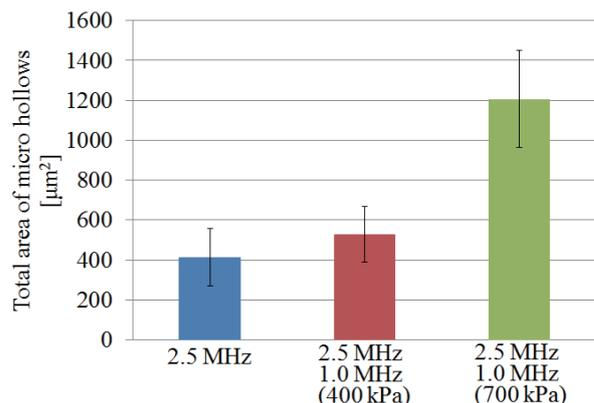
Fig. 5 Total area of micro hollows in high intensity US wave irradiation with 2.5 MHz single, 2.5 MHz + 1.0 MHz (400 kPa), and 2.5 MHz + 1.0 MHz (700 kPa), respectively.
