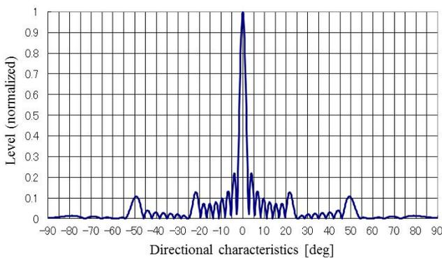
**Fig. 3 Focal position control with phase delay simulation (steering angle 0 degree focus point 100mm from module element surface)**
