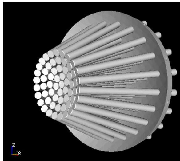
Fig.1 Schema of multi-elements module transducer
