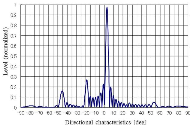
**Fig. 4 Focal position control with phase delay simulation (steering angle 2.862 degree focus point 100mm from module element surface)**
