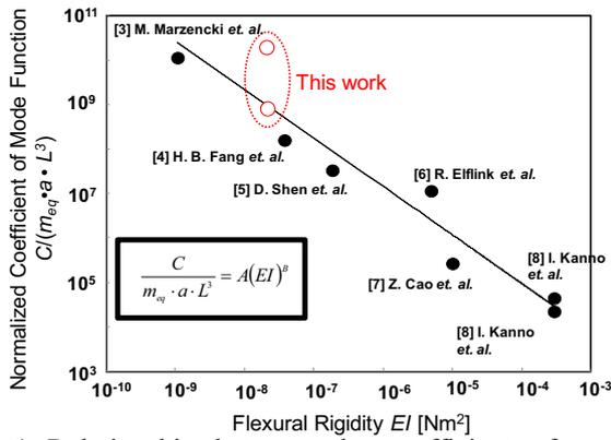
**Fig.1** Relationship between the coefficient of mode function  $C$  and the flexural rigidity  $EI$
