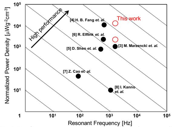
**Fig.3** Performance comparison based on the normalized power density
