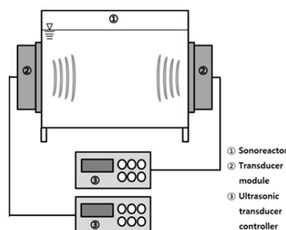
**Fig 1.** A schematic diagram of the experimental set-up.
