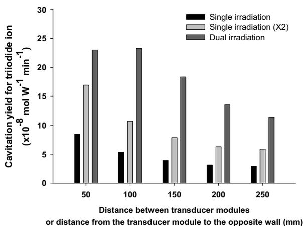
**Fig 2.** The variation of cavitation yields for single and dual irradiation in five distance conditions.
