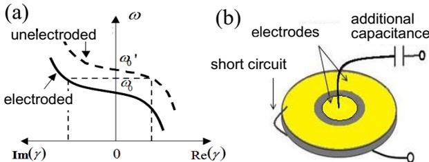
Fig.1 (a) Dispersion curve for a backward-wave-mode thickness vibration and (b) electrode configuration for energy trapping.
