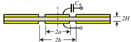
Fig. 2 Trapped-energy resonator with circular electrodes.
