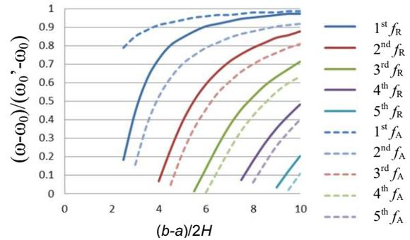
Fig. 6 Frequency spectra for variation in  $(b-a)/2H$  ( $a/H=1$ )
