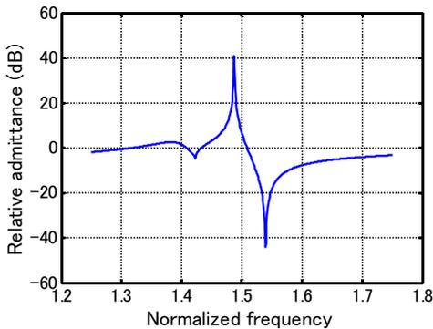
Fig. 5 Admittance characteristic when  $C_0/C_A=1$ .
