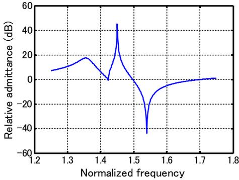
Fig. 4 Admittance characteristic without  $C_A$
