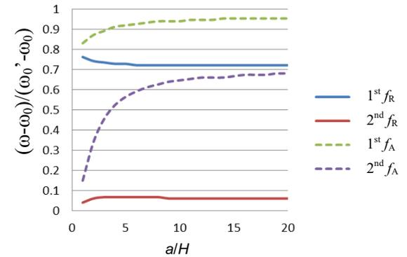
Fig. 7 Frequency spectra for variation in  $a/H$  ( $(b-a)/2H=2$ )
