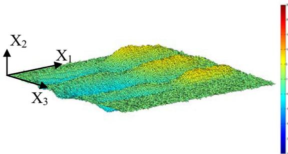
Fig. 4 Displacement of  $X_2$  axle of the 8MHz sample with “plaid” out-of-plane displacement. The directions of two nearby areas are opposite.
