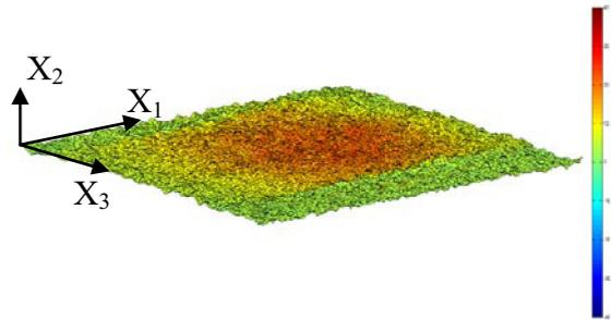
Fig. 6 Total displacement of the new design 8MHz sample. It shows that the out-of-plane mode are depressed.
