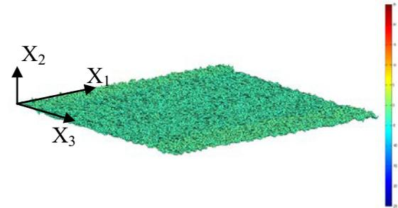
Fig. 7 Displacement of  $x_2$  axle of the new design 8MHz. The out-of-plane displacements are almost undetectable.
