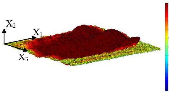
Fig. 3 Total displacement of the 8MHz sample with strong out-of-plane couple mode.
