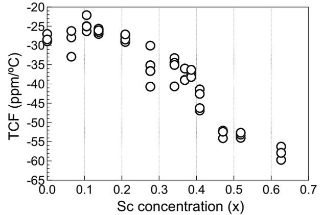
Fig. 3 TCF value of  $\text{Sc}_x\text{Al}_{1-x}\text{N}$  films
