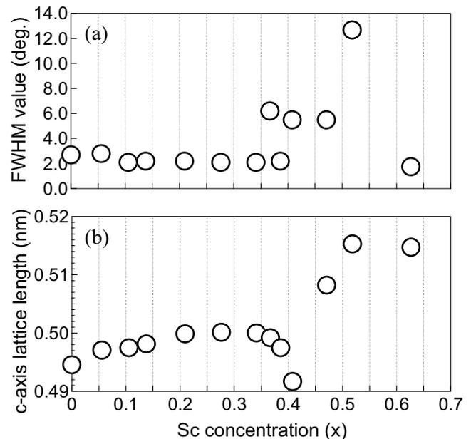
Fig. 1 (a) (0002) rocking curve FWHM value and (b) c-axis lattice length of the  $\text{Sc}_x\text{Al}_{1-x}\text{N}$  films
