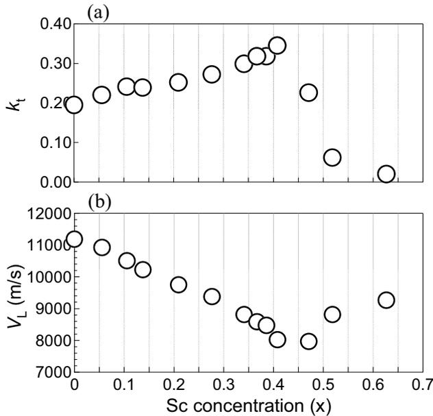
Fig. 2 (a) Electromechanical coupling  $k_t$  value and (b) longitudinal wave velocity  $V_L$  of the  $\text{Sc}_x\text{Al}_{1-x}\text{N}$  films
