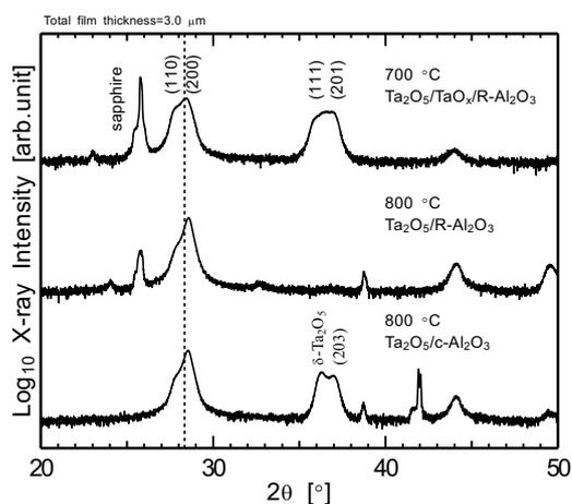
Fig. 1 XRD patterns of Ta<sub>2</sub>O<sub>5</sub> thin films deposited on TaO<sub>x</sub>/R-Al<sub>2</sub>O<sub>3</sub>, R-Al<sub>2</sub>O<sub>3</sub>, c-Al<sub>2</sub>O<sub>3</sub>.
