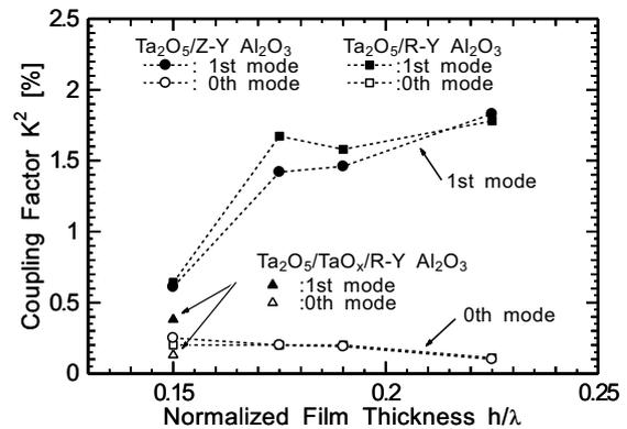
Fig. 4 Measured coupling factor K<sup>2</sup> values.
