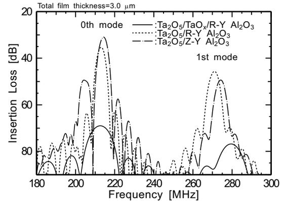
Fig. 3 Frequency responses of each sample with h/λ=0.15.
