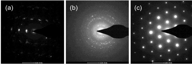
Fig. 2 TEM patterns of Ta<sub>2</sub>O<sub>5</sub> thin films deposited on (a) TaO<sub>x</sub>/R-Al<sub>2</sub>O<sub>3</sub>, (b) R-Al<sub>2</sub>O<sub>3</sub>, (c) c-Al<sub>2</sub>O<sub>3</sub>.
