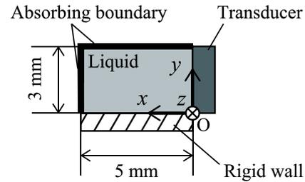
**Fig. 1** Simulation setup for sound wave propagation in liquid.
