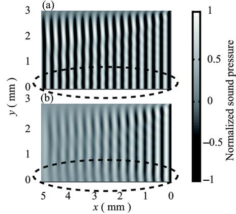
**Fig. 3** Sound pressure distribution; (a) in water and (b) in epoxy resin.
