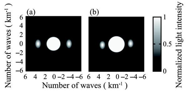
**Fig. 4** Diffraction pattern by sound pressure distribution; (a) with water and (b) with epoxy resin.
