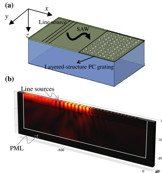
Fig. 3 (a) The PnC reflective grating for SAW. (b) The displacement field (amplitude of component  $U_z$ ) of 66 MHz SAW propagating toward the PnC grating.
