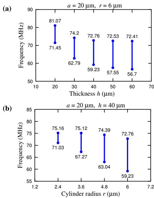
Fig. 2 The band gap ranges of layered-structure PnCs. (a) Varied layer thickness  $h$ . (b) Varied cylinder radius  $r$ .
