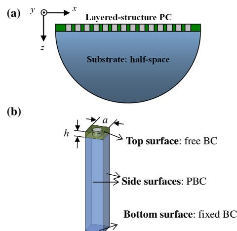
Fig. 1 (a) The schemas of a layered-structure phononic crystal. (b) The unit cell adopted in FE to analyze band of SAW.
