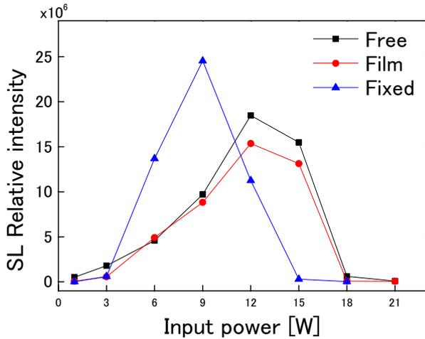
Fig.2 Power dependences of SL intensity for the three cases of boundaries.
