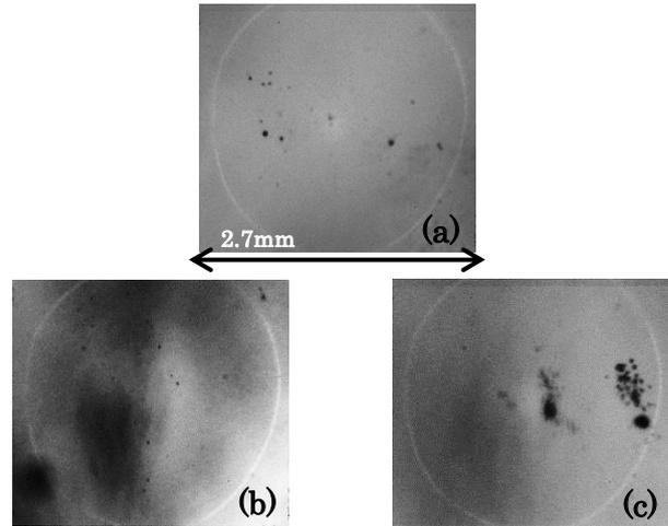
Fig.3 High-speed photographs of the acoustic bubbles for free-end boundary at (a) 3 W, (b) 12 W and 18 W at the speed of 64k fps.
