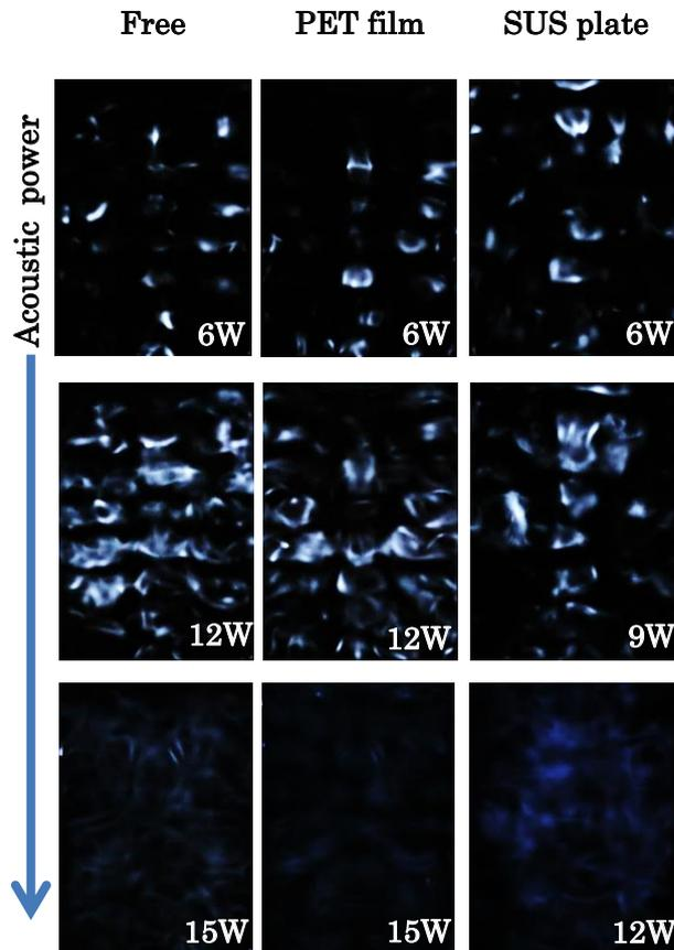
Fig.1 Power dependences of SL images for three cases of boundaries
