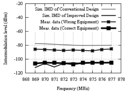
Fig.4 IMD measurement after optimization
