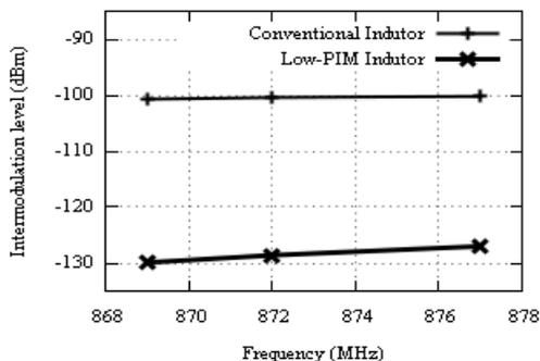
Fig.3 IMD measurement result of Inductors
