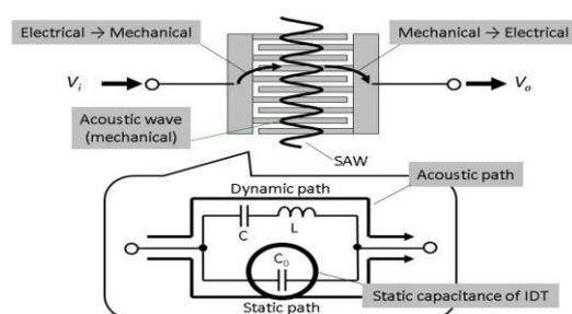
Fig.1 Possible origins of nonlinearity in SAW resonators
