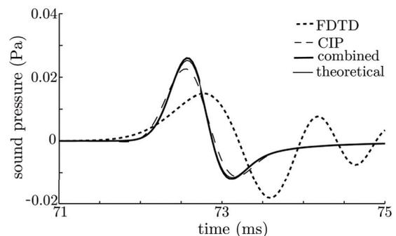
Fig.2 Sound pressure waveforms of direct wave.
