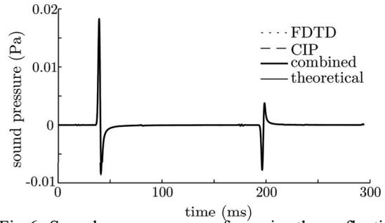
Fig.6 Sound pressure waveform in the reflective field with the longer pulse width.
