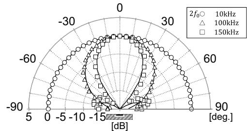
Fig. 5 Directivity patterns of radiated sound wave from the thermophone (solid lines indicate theoretical estimations assuming rectangular diaphragm).
