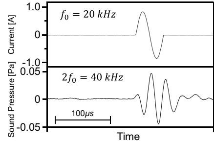
Fig. 2 Input current signal (top) and radiated sound wave (bottom) from the thermophone.
