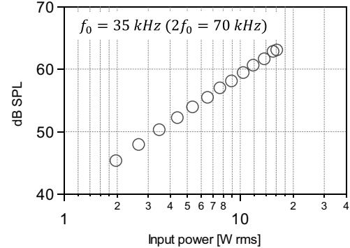
Fig. 3 Relationship between input power and sound pressure level of radiated sound wave from the thermophone.
