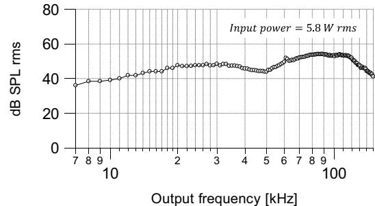
Fig. 4 Frequency characteristics of the thermophone.
