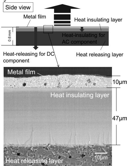
Fig. 1 Sectional view of Thermophone.
