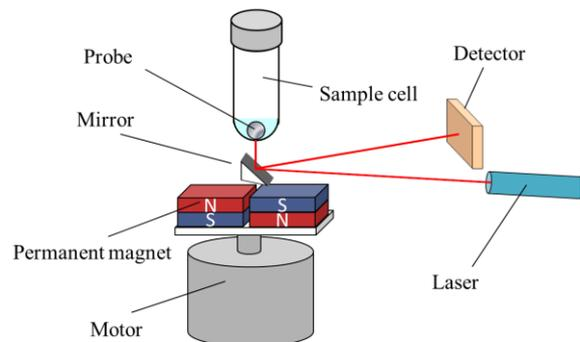
Fig. 2 Schematic view of a developed detection system
