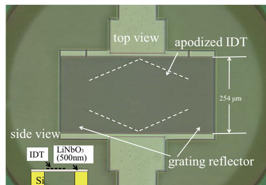
Fig. 2 High frequency SH<sub>0</sub> plate wave resonator fabricated on a 0.5μm thick 30° YX-LiNbO<sub>3</sub> plate (AR = 60%).
