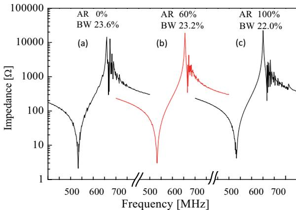
Fig. 3 Frequency characteristics of resonators with 3 kinds of apodization, (a) AR = 0%, (b) AR = 60% and (c) AR = 100%.
