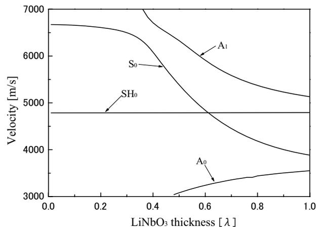
Fig. 1 Calculated phase velocity of plate waves on 30° YX-LiNbO<sub>3</sub> as a function of plate thickness.
