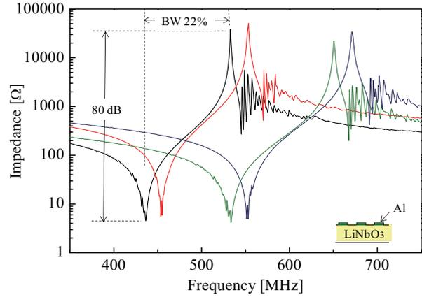
Fig. 4 Frequency characteristics of high frequency resonators shown in Table I.
