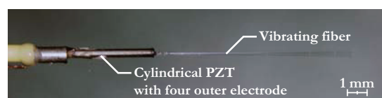
(a) Bending vibration of the optical fiber.
