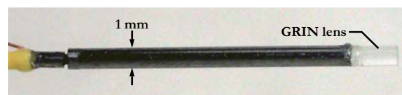
(b) Overview of the endoscopic optical scanner.
