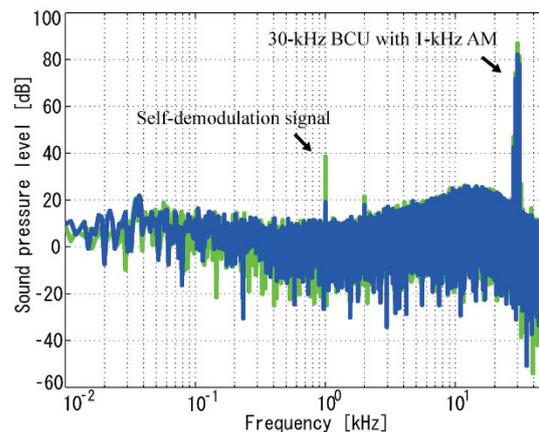
**Fig. 1.** Acoustic fields in the ear canal under a 30-kHz BCU stimulation with 1-kHz amplitude modulation before and after the occlusion of the ear canal.
