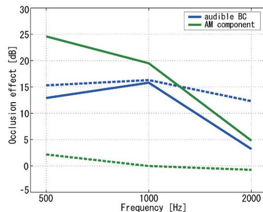
**Fig. 2.** The occlusion effects as sound pressure in the ear canal (solid lines) and subjective hearing threshold (dotted lines). The green lines represent for the self-demodulated signals and the blue lines for the signals derived from audible BC stimuli.
