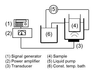
Fig. 1 Outline of experimental apparatus for ultrasonic irradiation at 500 kHz.
