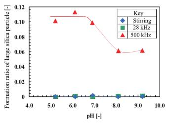
Fig. 5 Effect of solution pH on formation ratio of large silica particles for ultrasonic irradiation and stirring.
