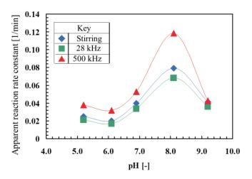
Fig. 3 Effect of solution pH on apparent reaction rate constant of silica monomer for ultrasonic irradiation and stirring.
