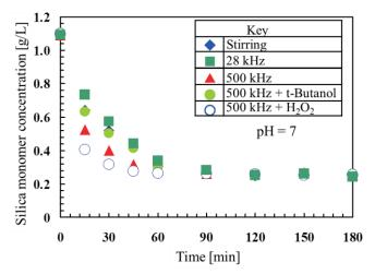
Fig. 2 Change in silica monomer concentration with time for ultrasonic irradiation, stirring and addition of chemical substances.
