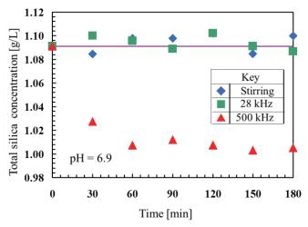
Fig. 4 Change in total silica concentration with time for ultrasonic irradiation and stirring.
