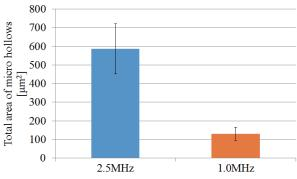
Fig. 2 Total area of micro hollows when high intensity US waves of 2.5 MHz and 1.0 MHz irradiate.
