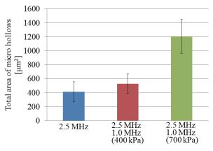
Fig. 5 Total area of micro hollows in high intensity US wave irradiation with 2.5 MHz single, 2.5 MHz + 1.0 MHz (400 kPa), and 2.5 MHz + 1.0 MHz (700 kPa), respectively.
