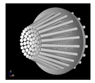
Fig.1 Schema of multi-elements module transducer
