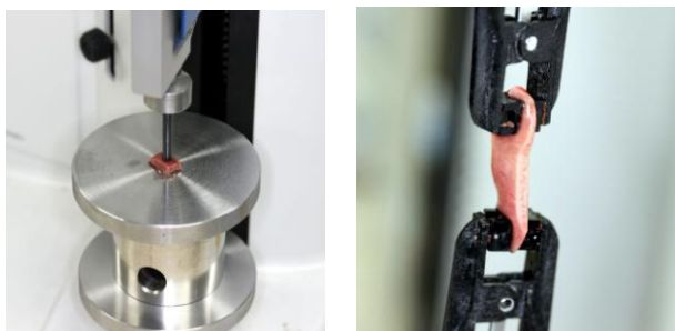
Fig. 3 Compressive test (left) and tensile test (right) of the rat liver
