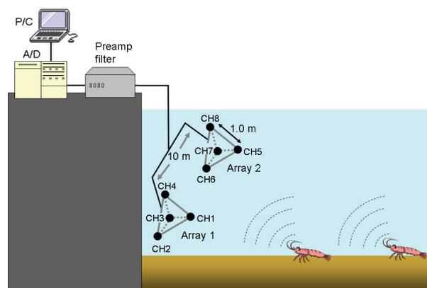
Fig. 1 Experimental setup for estimating source positions of biological transient noises.
