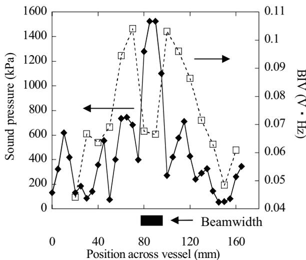
Fig.3 Variation in the BIV and sound pressure with position across the water vessel.
