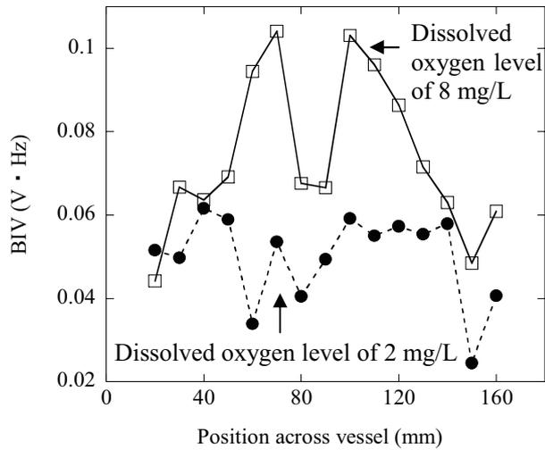
Fig.2 Variation in the BIV with position across the water vessel at DO level of about 2 and 8 mg/L.
