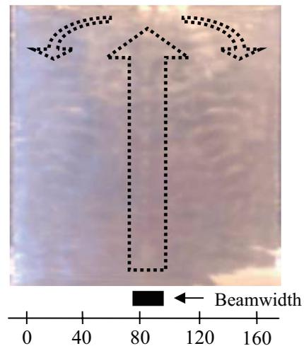
Fig.4 Photograph of acoustic streaming in water in the water tank of our ultrasound exposure system.
