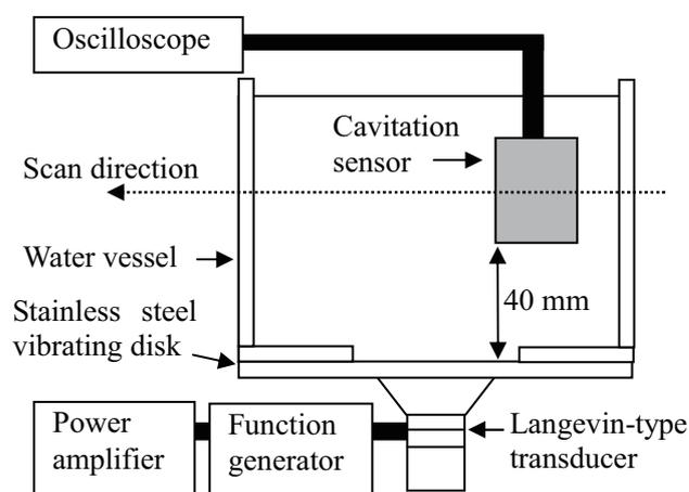
Fig.1 Experimental system for measuring the BIV.
