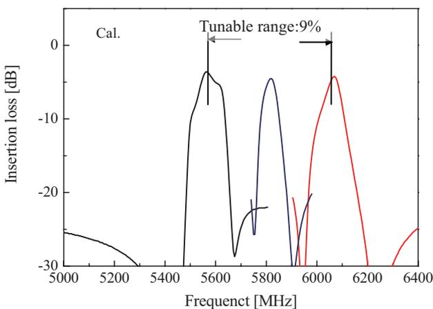
Fig.4 Frequency characteristics of tunable filter composed of ladder type.
