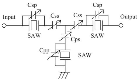
Fig.2 Ladder type filter to construct tunable filter.
