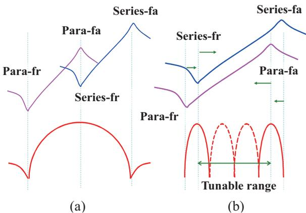
Fig.3. Frequency arrangement for ladder type filter (a) conventional arrangement and (b) arrangement for tunable filter.
