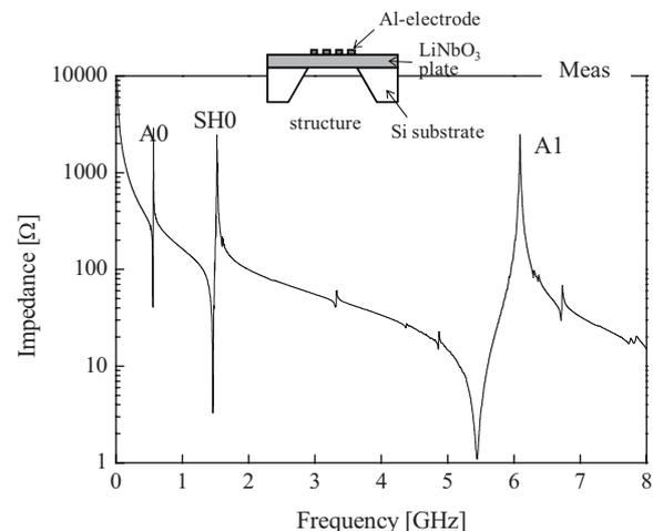
**Fig.1 Device structure and frequency characteristic of Lamb wave resonator on LiNbO<sub>3</sub> plate/Si.**
