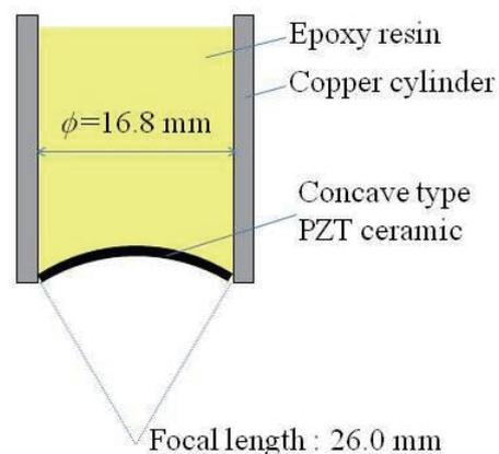
Fig. 1 Construction of a focusing ultrasonic transducer
