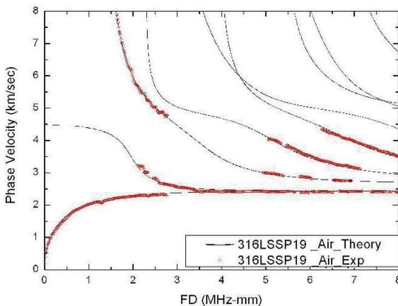
Fig. 3 Theoretical and experimental dispersion curves of 19.1% porosity
