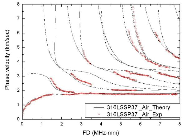
Fig. 4 Theoretical and experimental dispersion curves of 37.4% porosity
