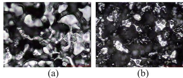
Fig. 1 Micrographs with (a)19.1% and (b)37.4% porosity.
