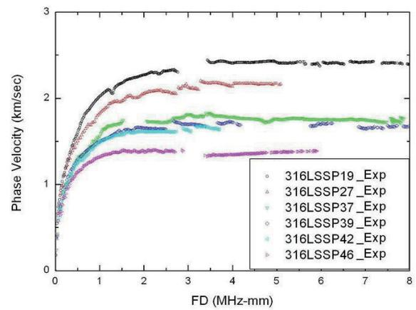
Fig. 5 Dispersion curve of A0 mode with different porosity samples
