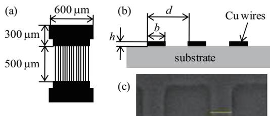
Fig. 1.(a) Schematic of the nanowire specimen. (b) Cross-section image of the specimen. (c) SEM image of the specimen. The bar indicates 300 nm.
