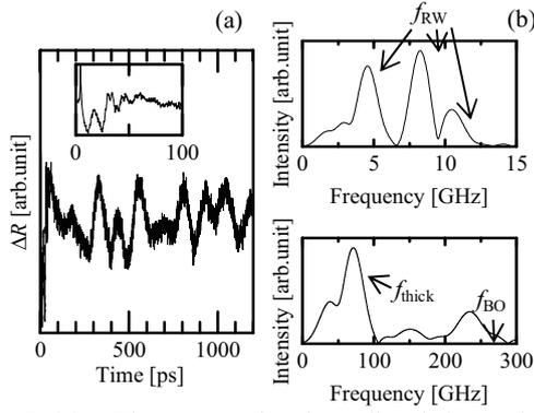
Fig. 2.(a) Time resolved reflectivity change observed for nanowires on Si substrate, and (b) their FFT spectra.
