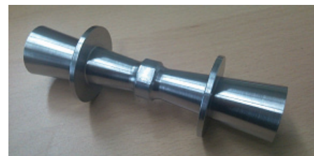
Fig. 2. Designed ultrasonic welding horn
