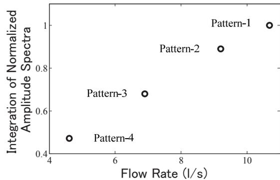
Fig. 4 Correlation between pipe flow rate and integration of the normalized amplitude spectra
