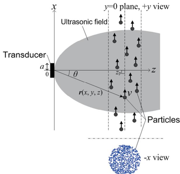
Fig. 1 Schematic diagram of the measurement setup
