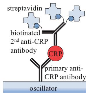
Fig. 1 Schematic of the mass-amplified sandwich assay. the weight of the 2<sup>nd</sup> antibody is increased by streptavidin molecules via biotin terminals.
