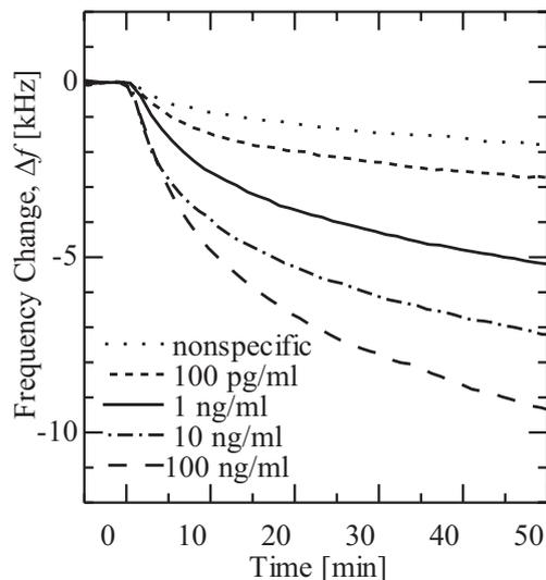
Fig. 3 Frequency changes caused by injections of the mass-amplification solution after injections of various concentrations of CRP solutions.
