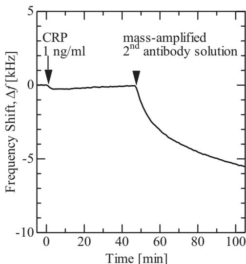
Fig. 2 Frequency change behaviors for the injection of 1 ng/ml CRP solution and the mass-amplified 2<sup>nd</sup> antibody solution.
